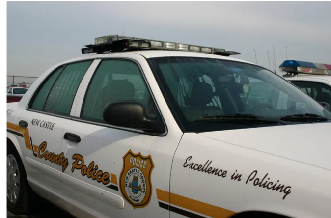
Cameras mounted on the front and side of this cruiser's light bar scan license plates. The Community News
